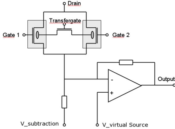
Fig. 4. Simplified scheme of the RNDR device and the readout setup. The I/V converter defines a common Source potential for both DEPFETs ( $V_{virtual\ source}$ ). By turning one DEPFET off during the other one is on and vice versa enables the readout of both DEPFETs with only one readout node.
