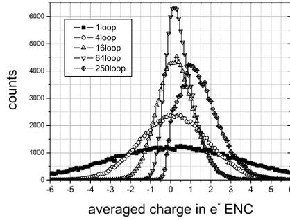
Fig. 2. Simulated noisepeaks of a RNDR detector with  $\sigma = 3.3 e^- ENC$  for different numbers of readouts (1, 4, 16, 64 and 250), for a given leakage current of  $i_l = 0.0003 e^- / (\mu s \cdot Pixel)$  and a readout time of  $t_{loop} = 34 \mu s$  and an integration time of  $t_{int} = 414 \mu s$ . For the given parameters, the lowest readout noise can be achieved with 64 loops.
