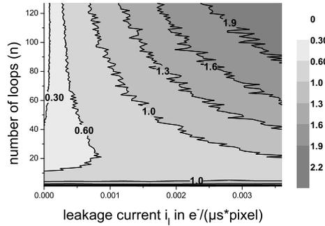
Fig. 3. Monte Carlo map showing the noise in  $e^- ENC$  as a function of the leakage current vs number of loops. The isolines show the minimum achievable noise in  $e^- ENC$ , Parameters:  $\sigma = 2.0 e^- ENC$ ,  $t_{loop} = 34 \mu s$ . To see the pure impact of the leakage current to the resolution an integration time of only  $t_{int} = 1 \mu s$  was used.
