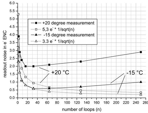
Fig. 5. Theoretical expectation and measured noise in  $e^-$  ENC vs number of transfer loops. For two different temperatures of +20 degree and -15 degree measurements are shown, the monotonously falling curves show the respective theoretical noise limits given by eq. 1.
