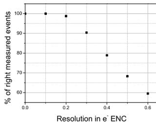
Fig. 6. Probability to measure the right number of electrons for different resolutions. With a resolution of  $\sigma_{end} = 0.3 e^-$  ENC it is possible to determine the right number of collected electrons with a probability of 90 percent.
